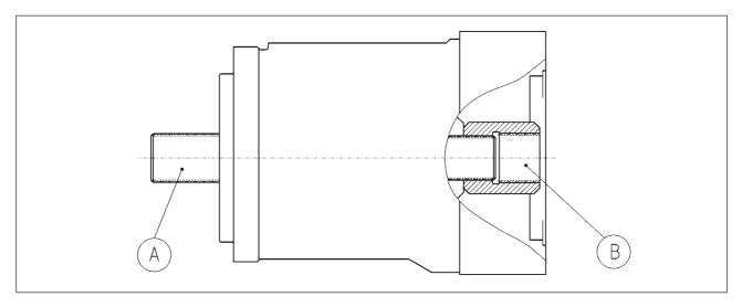
The diagram Torque transmission of HMF / A / V / R-02 shows the output side A and the PTO through-shaft B of a motor. The information on the following pages refers to
