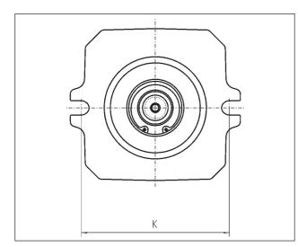
2-hole flange with 4 additional bolt holes
