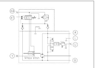
Regulating motor with pneumatic  $V_{max}$  override control
