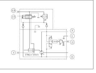
HMR-02 with electric  $V_{max}$  override control and signal selection for pressure regulator
