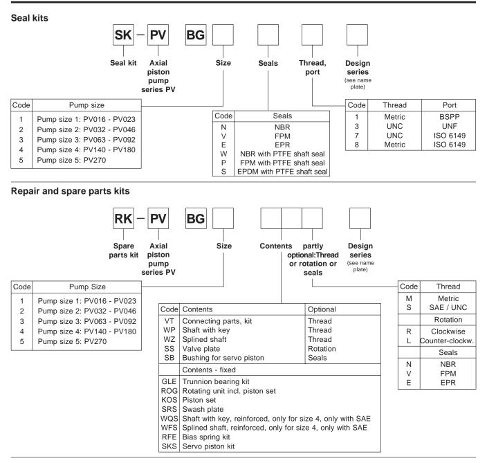
Repair and spare parts kits for adjustable displacement limiter
