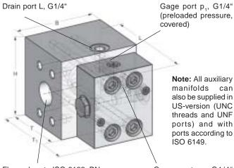
Flanged ports ISO 6162: DN, PN; fits to PV frame size BG; threads: M
