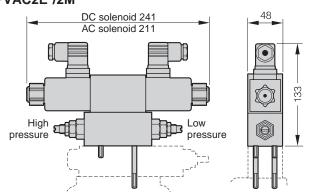
2-pressure relief valve, electrical selection and unloading, mounted on compensator type R or F  $\,$
