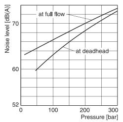
Typical sound level for single pumps, measured in unechoic chamber according to DIN 45 635, part 1 and 26. Microphone distance 1m; speed: n = 1500 min-1.
