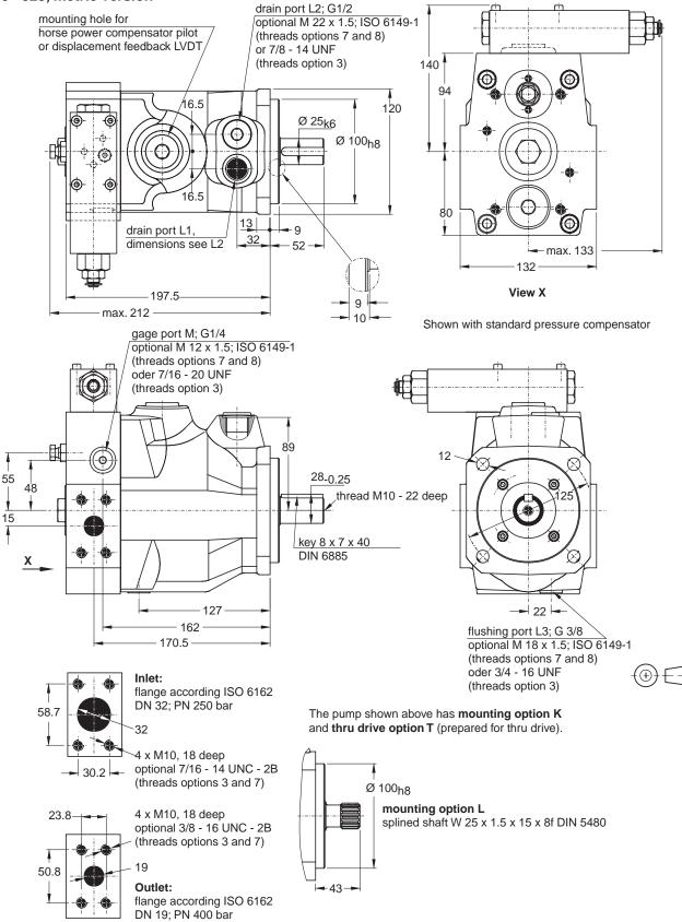
For further information about flanges see catalogue No. 4039/UK "Pressure Hydraulic Flanges" (on request). Shown is a clockwise rotating pump. Counter clockwise rotating pumps have inlet, outlet and gauge ports reversed. PI PVplus UK.PMD RH
