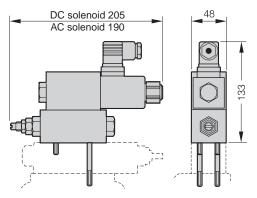
Pressure relief valve, electrical unloading, mounted on compensator type R or  $\ensuremath{\mathsf{F}}$
