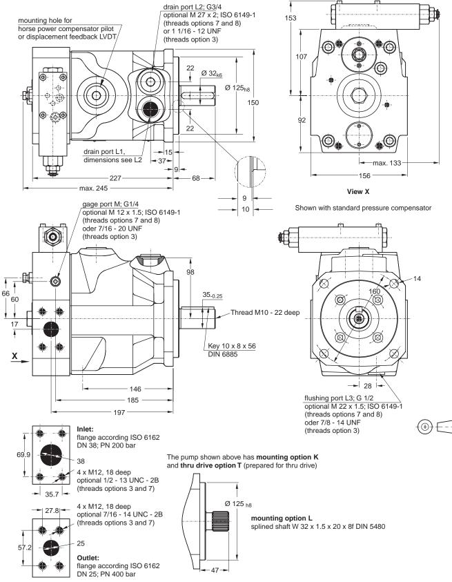
For further information about flanges see catalogue No. 4039/UK "Pressure Hydraulic Flanges" (on request). Shown is a clockwise rotating pump. Counter clockwise rotating pumps have inlet, outlet and gauge ports reversed. PI PVplus UK.PMD RH
