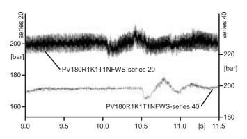
**Figure 2:** Comparison of the pressure pulsation in a system with 6 old PV pumps versus the same system with 6 PVplus pumps. The pulsation reduction effect of the precompression volume is evident.
