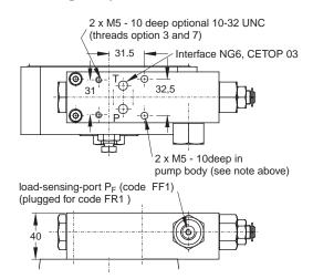
Proportional p-Q-compensator, code FPR (for code FPV lower valve only without interface)
