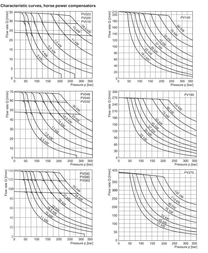
The diagrams shown are only valid for the following working conditions: Speed : n = 1500 rev/min Fluid t = 50°C Temperature Viscosity
