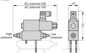
2-pressure relief valve, electrical selection, mounted on compensator type R or  $\mathsf{F}$
