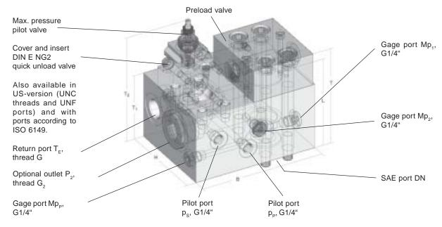
Flange ports ISO 6162; DN, PN; fit to PV, frame size BG; thread M
