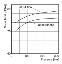
All data measured with mineral oil viscosity 30 mm<sup>2</sup>/s (cSt) at 50°C.
