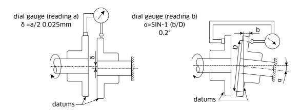
For engine drives a split type pinch bolt drive flange and flexible coupling is recommended.
