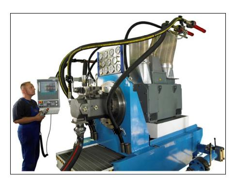
Advanced pump repair testing rig
