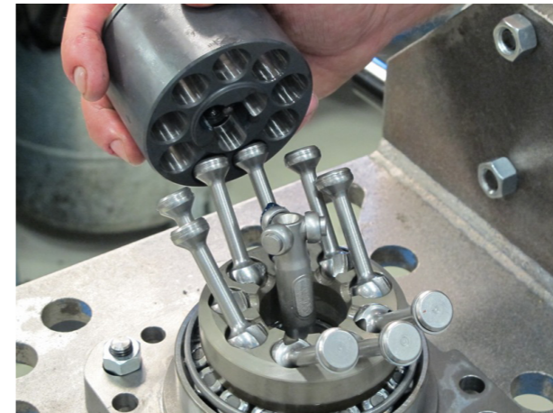
48. Assemble the cylinder barrel. Make sure that all rollers are in place.
