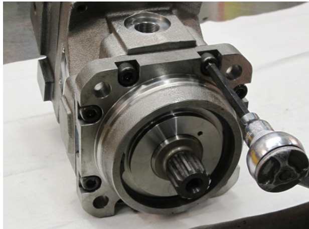
55. Assemble the screws and torque the screws to 65±10 Nm for V12-60/80 and 105±20 Nm for V12-110/160.
