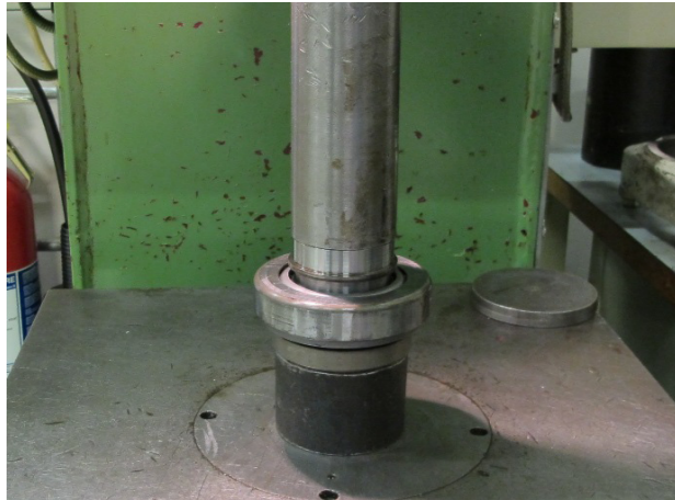
1. Press down the big tapered roller bearing and the inner ring for the roller bearing in two steps. Note! On V12-060 there is a distance between the bearings.
