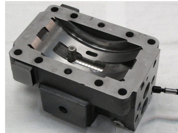
25. Assemble the set screw with the flat end.
