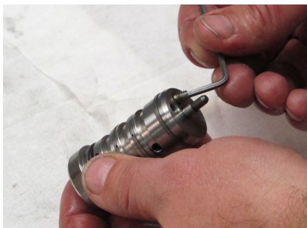
32. Assemble the nozzles and torque them to 1,2 \pm 0,2 Nm.
