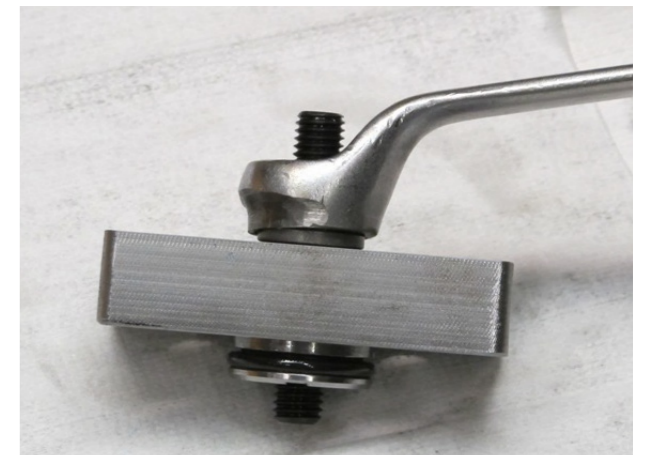
12. Assemble the displacement setting screw, seal nut and the O-ring.
