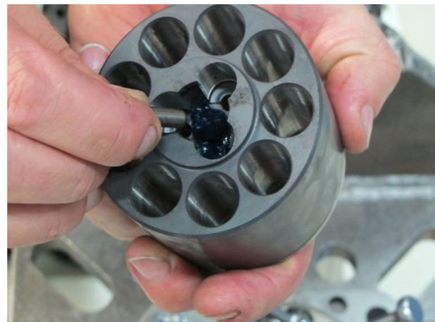
47. Assemble the support pin. Use a lot of grease to keep it in place.
