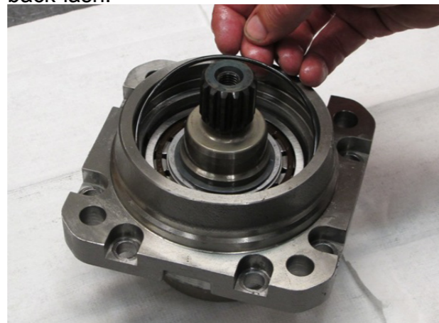
6. Assemble the O-ring.
