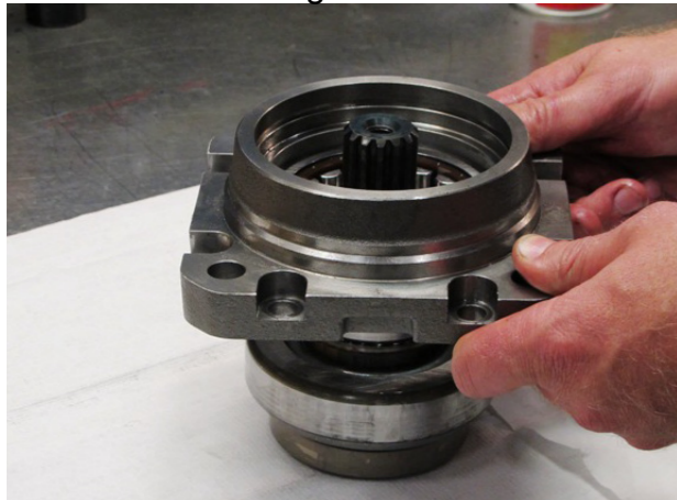
2. Press down the roller bearing with the text upwards into the flange and assemble it on the shaft package.
