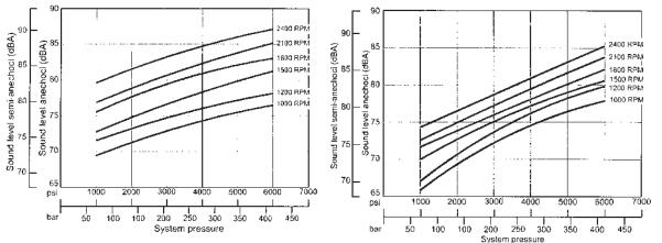
**Note:** Pump acoustical data was determined in accordance with ANSI/B93.71M, Hydraulic Fluid Power Pumps test code for the determination of airborne noise levels. Semi-anechoic values are presented according to the standard. Anechoic values are calculated for comparison with DIN 45635, part 1. The DIN standards measures sound levels over different surface areas so comparisons are not exact.
