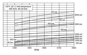
VOLUMETRIC EFFICIENCY @ FULL STROKE
