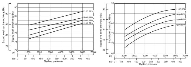
**Note:** Pump acoustical data was determined in accordance with ANSI/B93.71M, Hydraulic Fluid Power Pumps test code for the determination of airborne noise levels. Semi-anechoic values are presented according to the standard. Anechoic values are calculated for comparison with DIN 45635, part 1. The DIN standards measures sound levels over different surface areas so comparisons are not exact.
