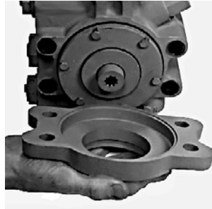
Remove Auxiliary Pad Adapter
