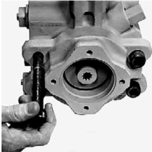
Remove Auxiliary Pad Adapter Screws
