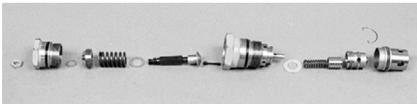
90000278 Multi-Function Valve Cartridge Components (Earlier production)
