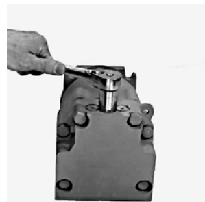
90000342 Remove Shim Charge Relief Valve
