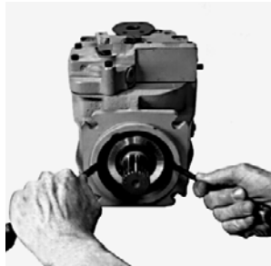
90000271 Remove Seal Carrier
