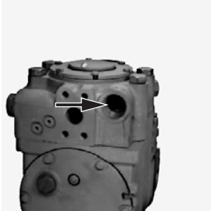
Charge Pump Inlet
