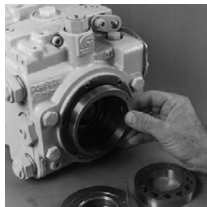
Install Gerotor Assembly Outer Ring
