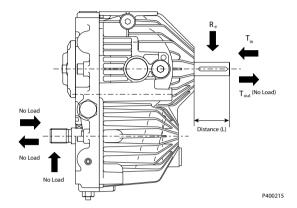
The maximum shaft thrust in (**Tin**) of input shaft is 18% of allowable radial road (**Re**) of the input shaft. The shaft thrust out (**Tout**) of the input shaft should be no load. The radial and thrust load of the output shaft should be no load.
