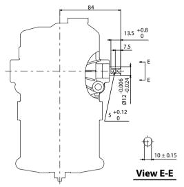
Right-hand side viewing from input shaft (when pump located upside) Option Code : R
