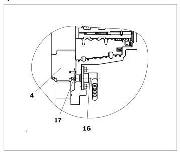
A Hall-effect speed sensor (16) may be fitted as an option, giving a two-channel output of phase-displaced square waves, and enabling detection of speed and direction. A toothed target disc (17) is fitted to the motor cylinder block (4), and the sensor, fitted to a port in the rear case, produces a pulse on each channel as each tooth passes in front of it. The frequency of the pulses is proportional to the rotational speed.
