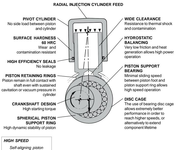
Piston support bearing Piston retaining rings
