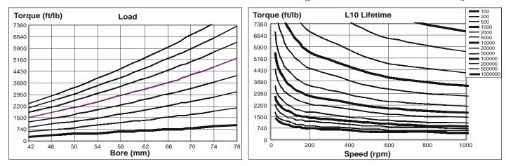
**BEARING OPTIONS** Special higher capacity spherical roller bearing (option GX) - the lifetime is approximately 2.29 times the equivalent lifetime given in the graph.
