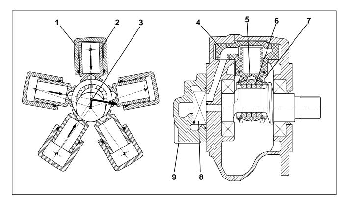
**Pivoting cylinder:** the cylinder (1) remaining aligned with the eccentric of the crank (3), eliminates side loading between the cylinder and piston (2). The articulation of the cylinder-piston assembly is achieved with large diameter trunnions (4) ensuring low specific loads.
