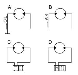
A: Freewheeling with oil circulation: this condition is acceptable for low speeds only. At high speeds the motor inlet must be pressurized to prevent noise due to cavitation. B: Freewheeling with air circulation: this condition is ideal for high speed freewheeling applications; transition from or to normal operation must be effected at low speed and pressure while the pistons are emptied or filled with oil.
